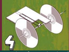
Step 4: Attach the wheels. Take a washer for each wheel and connect the washer to the CD with poster putty. Do a really good job of attaching them together. Use some of the putty around the skewer to create a bump in the skewer to keep the wheel in place.
