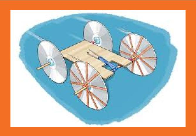
Step 5: Choose a rubber band and tape it to the cardboard opposite the notched out axle side. Stretch the rubber band to the other axle with the tape catch. Wrap the rubber band over the tape and begin to wind the axle up. The rubber band should get tighter and tighter around the axle. When you let it go the car should fly forward.
